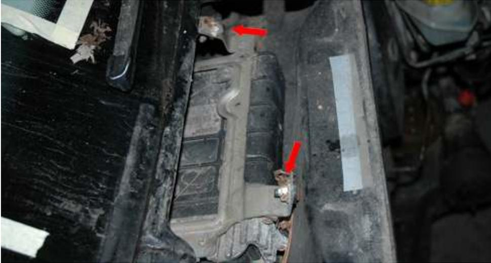
After you remove the two bolts, slide the bracket towards the passenger side then out. Next, push/pull the harness connector up.
