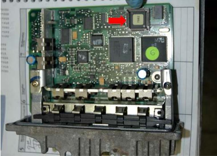
Carefully use a pick or a thumbtack to remove the old chip
