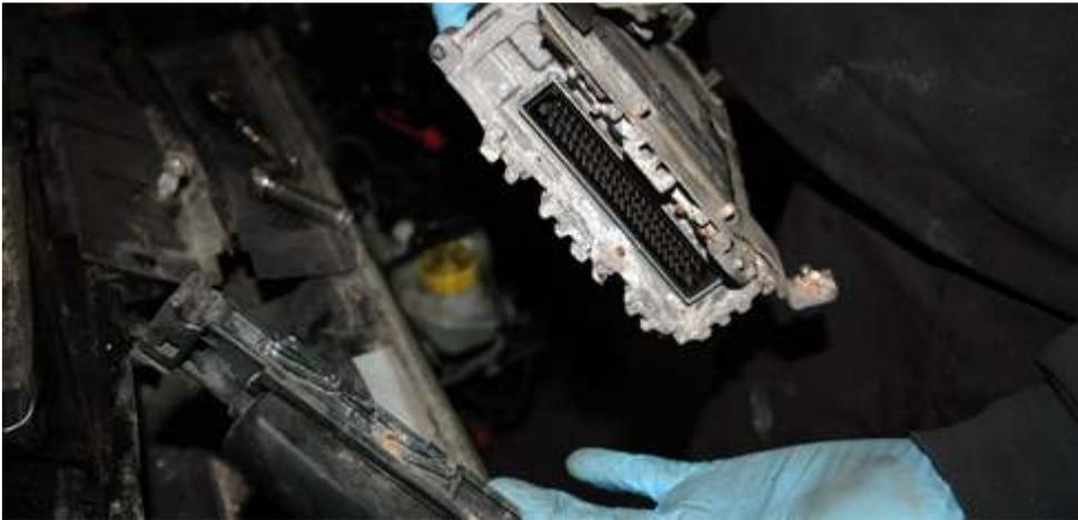
Remove (4) screws that attach the bracket to the ECU
